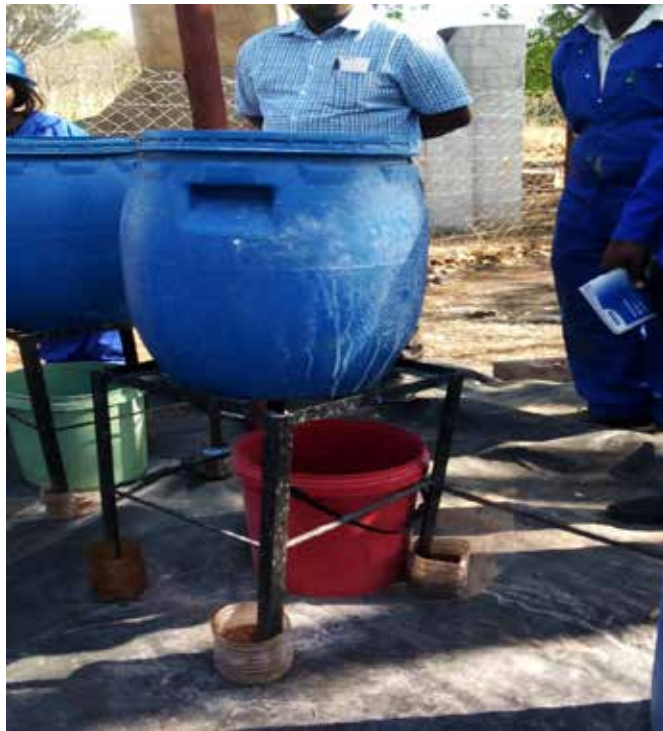
Figure 1: DDT Filtration system mounted on the stand
