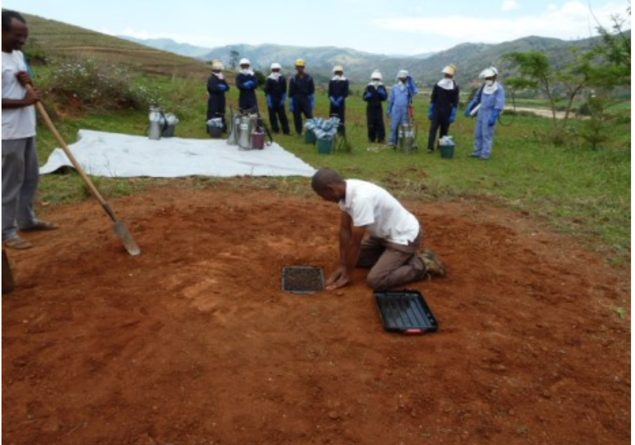
Figure 2: Installation of the receiving bucket in the ground
