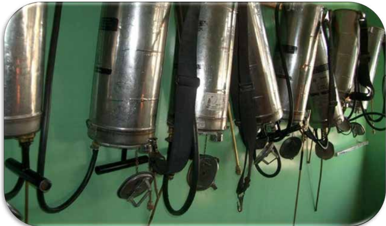
Sprayer pumps stored upside down to drain water.
